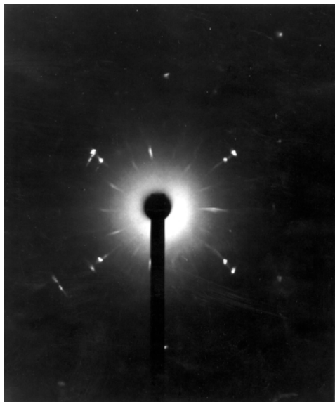
Fig. 3 Transmission X-ray Laue photograph of the single crystal \text{Ag}_2\text{Se} as in Fig. 2(c).
